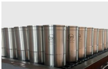
We have laser marking machine for traceability and mark logo. Neat, clean & indelible marking of Logos & Part no. are marked which doesn't produce stress or change in physical properties of materials. Marking are proof from chemical, water, Oil Grease and fuels.
