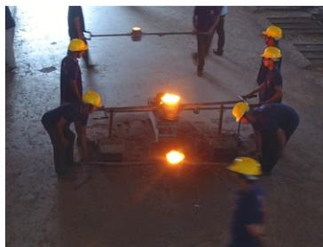
Melting process is carried out by 2 crucibles by dual track induction melting furnaces with continuous monitoring melting process by Pyrometers and Spectrometer. The most commonly used melting system is the induction crucible furnace. The induction crucible furnace has a crucible which is heated by an induction furnace coil surrounding the crucible.
